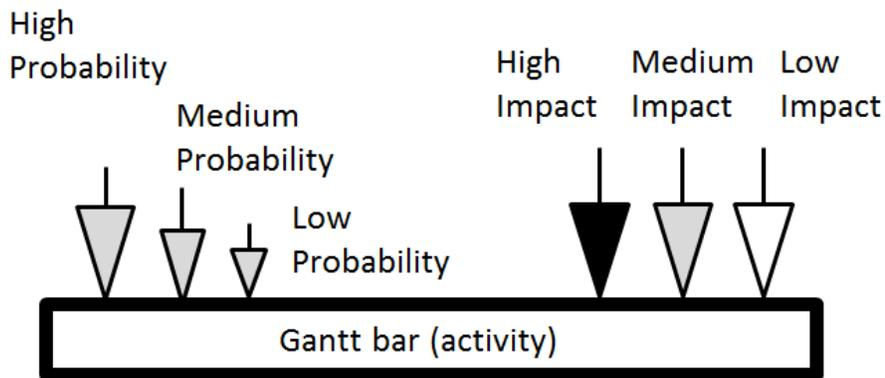
Figure 3. Showing risks with different probabilities and impacts
